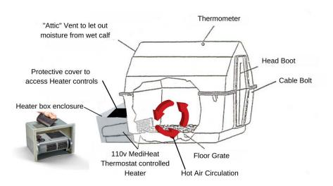
Hot air circulates around the calf to raise the body temperature and dry out the calf. The head boot allows the calf to breathe fresh air
